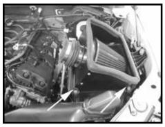
Step 8 Install the heat shield making sure that the tabs on the heat shield are inserted into the lower factory air box slots. With the heat shield located into the slots, using the 2 factory clips from the air box, clip the heat shield into position.
